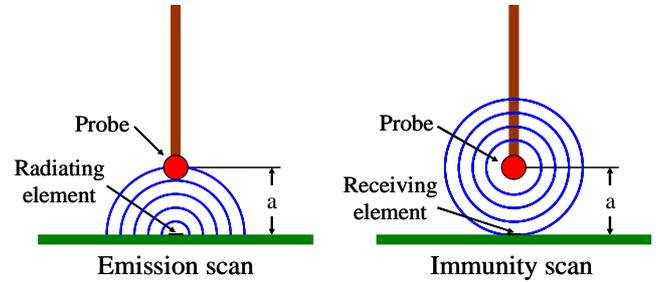
Fig. 6. Field received and radiated from a probe
